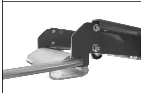
5. Fit the connecting bars (16) to one of the frame assemblies as shown and fix in place using hex bolts (11), flat washers (12), spring washers (13) and nuts (14).
